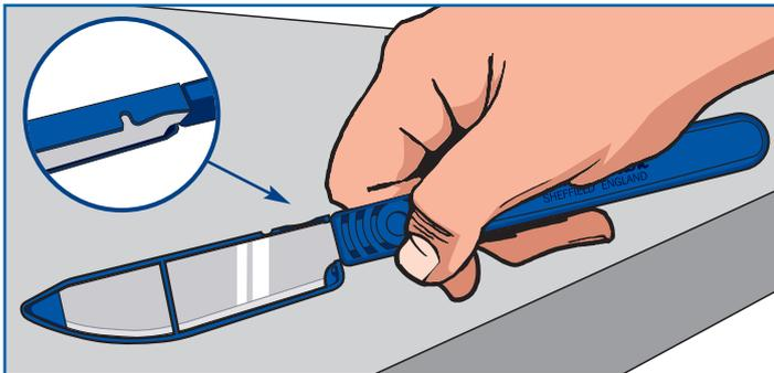
**1** Preferably place the Disposable Scalpel over a stable flat surface and identify the guard remover impression highlighted in the illustration.
