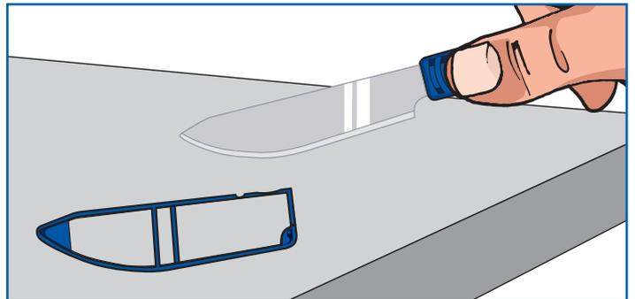
**4** The blade is now fully exposed and the Scalpel is ready for use.
