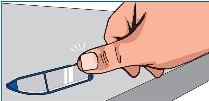
**2** With your thumb located in the guard remover press downwards with your thumb and the guard will release with an audible click.
