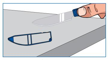
**4** The blade is now fully exposed and the Scalpel is ready for use.
