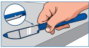
**1** Preferably place the Disposable Scalpel over a stable flat surface and identify the guard remover impression highlighted in the illustration.
